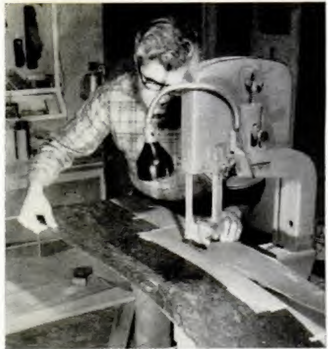
OAK FRAMING PIECES are cut to size on table saw. The new tongue must be formed on the cutoff side
